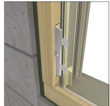
Figure 12: Using storm brackets
